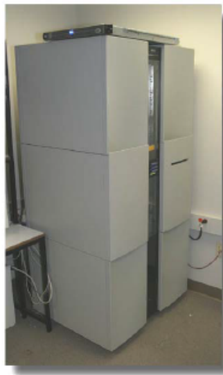
Juke Box Storage Unit at Larson Manufacturing used to store many of the 15,466,499 documents in their system.
